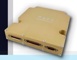
PRO-2 is a low-profile OBC designed for various missions, where intensive processing is not a primary requirement. However, it offers the capability to deliver up to 200 DMIPS on its ARM Cortex-M3 core if processing demands arise. Equipped with a versatile range of interfaces—including GPIO, ADC, CAN, RS232, RS422, and optional Ethernet—OBC-PRO-2 provides robust support for various mission-critical functions while maintaining a compact & efficient design.
